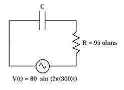
b.) We need to determine the capacitance C. We know the capacitive reactance is  $X_c = 1/(2\pi vC)$ , and we know that when the frequency is 300 hertz,  $X_c$  equals 198.4  $\Omega$  (from above). Manipulating the  $X_c$  expression, then plugging in, we get:
